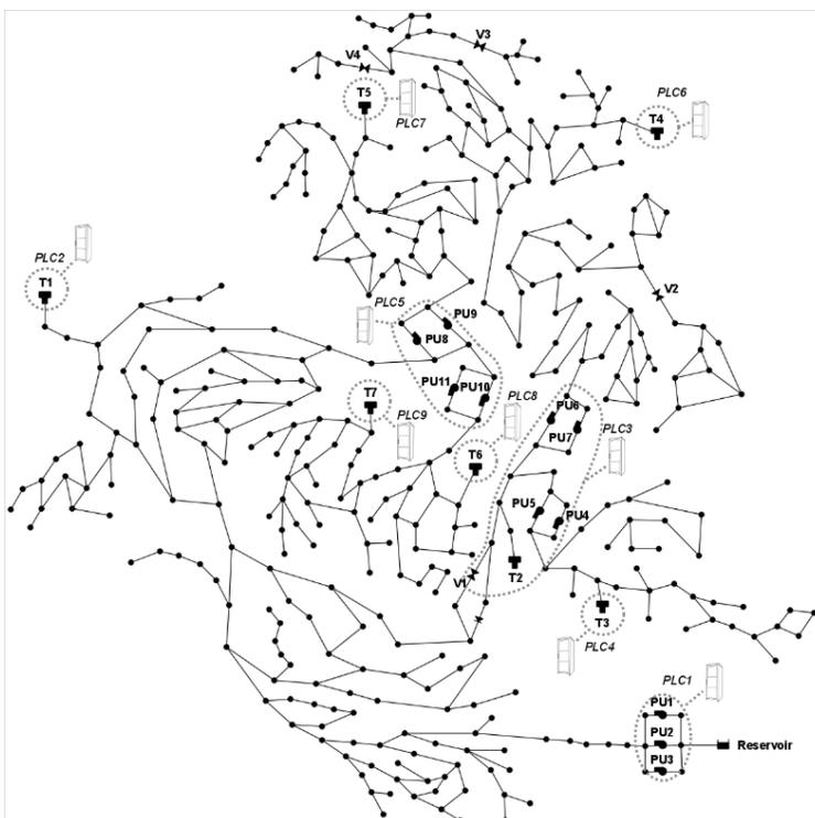
Figure 1: Graphical representation of C-Town water distribution system.
